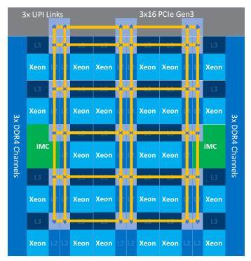
In the Intel® Xeon® Scalable processor platform Intel® Mesh Architecture with up to 28 cores (per processor), the Last Level Cache (LLC), six memory channels, and 48 PCIe\* channels are shared among all the cores, giving access to large resources across the entire die and creating dynamic scalability without sacrificing performance.
